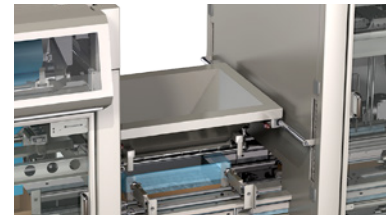
Demountable hopper for easy cleaning
