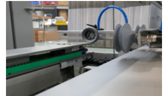
Box is clamped at three sides
