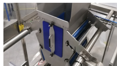
Opening door to the hoppers for cleaning access
