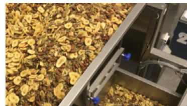
Diverter plate for coarse and fine filling
