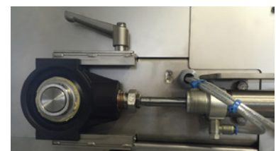
Demountable belt with quick release
