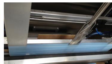
Bag stretching with integrated decuffer control
