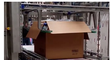
Combined bag closer with case closing module (optional)
