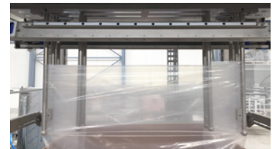
Regussetting before sealing
