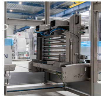
Tiltable infeed conveyor for easy cleaning
