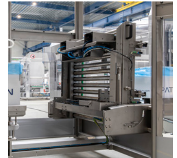
Tiltable infeed conveyor for easy cleaning
