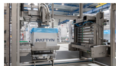
Tiltable infeed conveyor for easy cleaning
