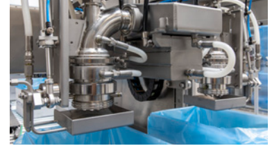
90° curved valve with drip catcher
