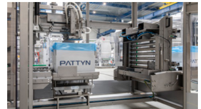
Tiltable infeed conveyor for easy cleaning
