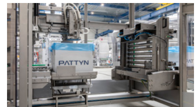
Tiltable infeed conveyor for easy cleaning
