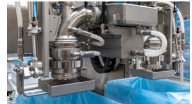
90° curved valve with drip catcher
