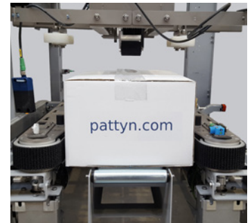
Robust side belts, driven by 2 motors
