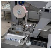
Easy tape loading system for upper taper
