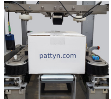
Robust side belts, driven by 2 motors
