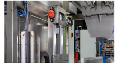
Box lift system to reduce drop distance
