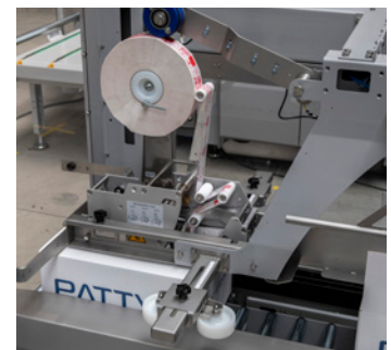
Easy tape loading system for upper taper
