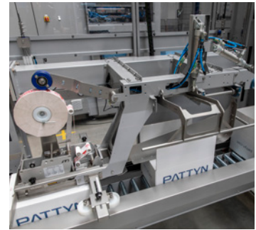
Pneumatic driven long flap folding
