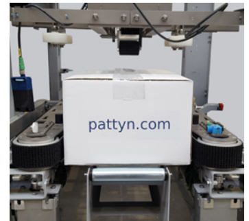
Robust side belts, driven by 2 motors
