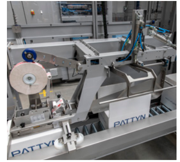
Pneumatic driven long flap folding
