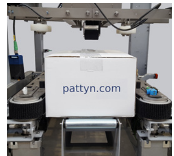
Robust side belts, driven by 2 motors
