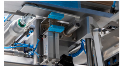
Robust spoons & mechanical grippers
