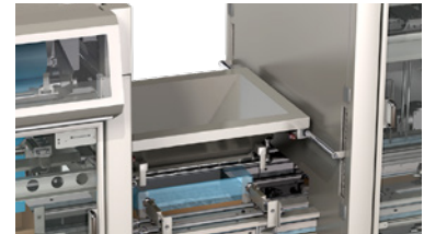
Demountable hopper for easy cleaning
