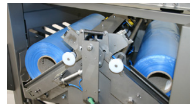
Automatic film roll exchange
