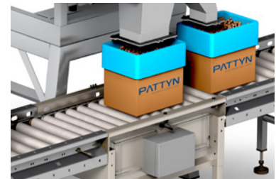
Fine dosing in separate weigh hopper for minimum after-fall.
