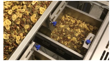
Diverter plate for coarse and fine filling
