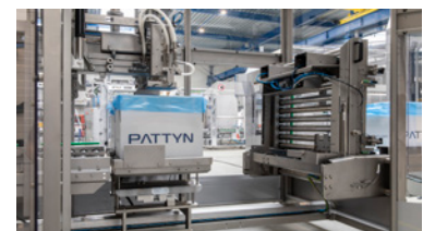
Tilttable infeed conveyor for easy cleaning
