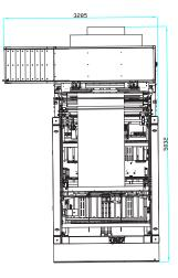
Min. machine height 2360 mm Max. machine height 3560 mm
