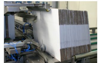
Failsafe carton separator
