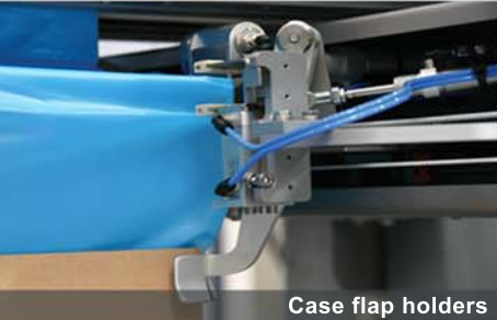
Mechanical grippers & spoons with air nozzle
