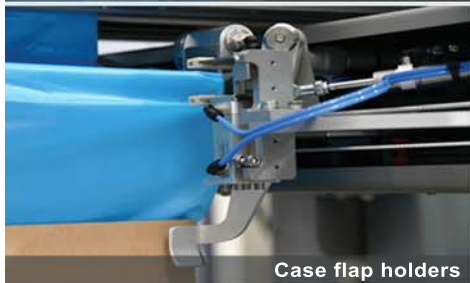
Mechanical grippers & spoons with air nozzle
